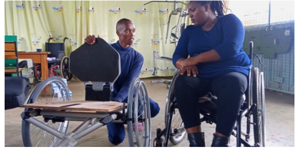
Figure 2 Technician showing the users how to remove and fold the seating unit
